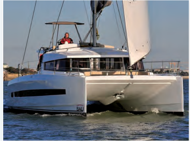
The design and construction of the ski-shape forward is really noteworthy, and the bridgedeck clearance is comparable with the competition. Fine-entry bows, reasonable weight loading, overall intelligent structure and hulls give great results on the water.
