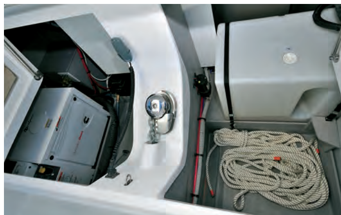
→ Beneath the forward seats are the tanks, the generator (if air-con is fitted) and the ground tackle. The chain locker is vast, so no danger of the chain piling up.
