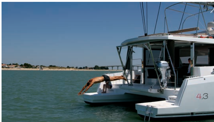
↑ The folding aft platform is a real bonus: neat stowage for the dinghy, and when opened up at anchor, it offers an area entirely open to the sea.
